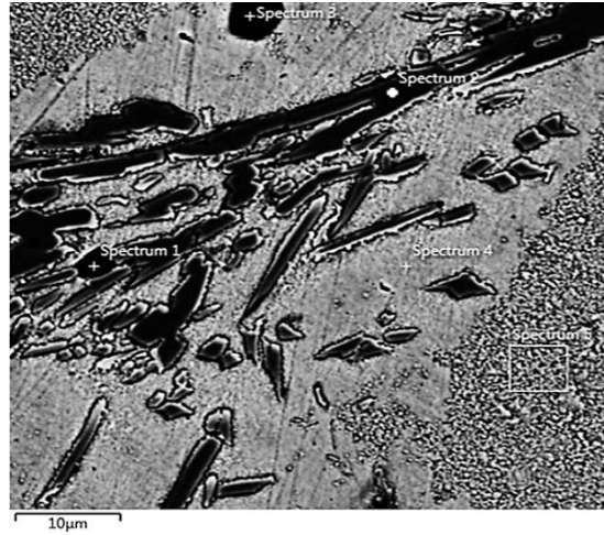
Figure 4 SEM BSE image and EDS map of precipitates formed at the grain boundary
