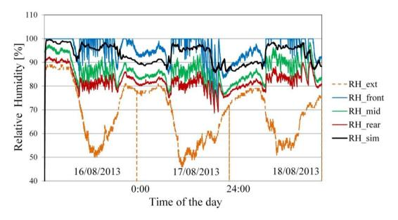
Figure 5 The simulated relative humidity compared to real plant data
