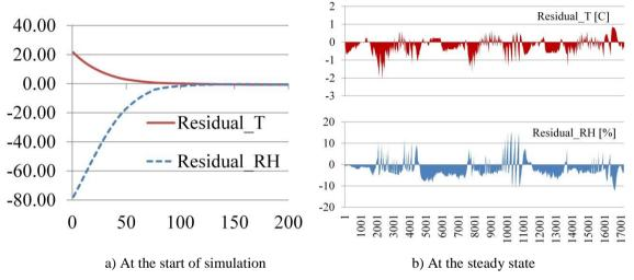
Figure 6 Residual plots of temperature at the rear part and relative humidity at the front part of the poultry house
