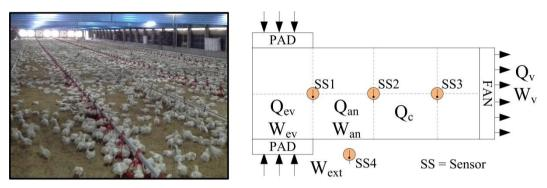
Figure 1 Heat and moisture components of the closed poultry house with tunnel ventilation
