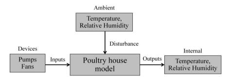
Figure 3 Feedforward climate control diagram of the poultry house
