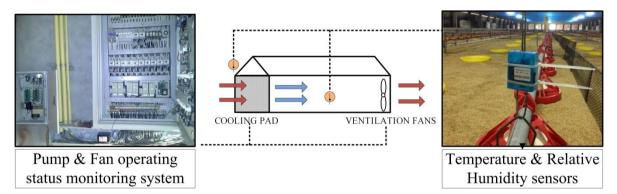
Figure 2 High-level block diagram of the air sensor set and the data logger
