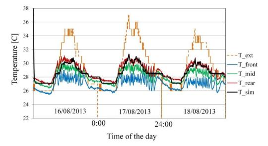
Figure 4 The simulated temperature compared to real plant data
