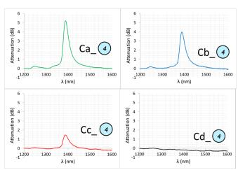
Fig. 6. Attenuation vs.  $\lambda$  for fibers into cables Ca, Cb, Cc, Cd after irradiation 3; cables in position 3 (22°C; 4.5 kGy/h; 1.8 MGy). To erase the attenuation due to connectors, all graphs are normalised to cancel attenuation at 1200 nm, where RIA is expected to be very low on such short lengths.
