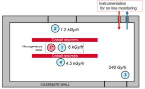
Fig. 1. Diagram of the POSÉÏDON casemate with positions used, and associated dose rate. 1\* simply differs from 1 by a higher temperature (about 80°C instead of room temperature).
