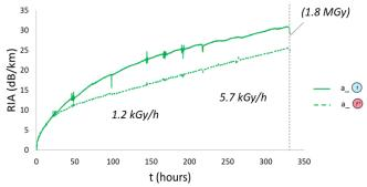
Fig. 3. RIA@1550 nm vs. time for fiber a during irradiation 1 in configuration ① (22°C) and ②(80°C). The dose rate is 5.7 kGy and the cumulated dose is 1.8 MGy at the end of irradiation.
