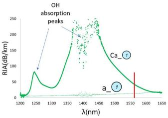
Fig. 5. RIA spectrum for fiber a and cable Ca at the end of irradiation 2 (cumulated dose: 1.5 MGy), in position  $\bigcirc (30^{\circ}\text{C}/5 \text{ kGy/h})$ .
