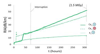
Fig. 4. Irradiation 2: RIA@1550 nm vs. time for fiber a in position (see Fig. 1), at room temperature (RT), and cables Ca, at RT (position and in oven at 80°C (position b). The dose rate is about 5 kGy/h. At the end of irradiation, the cumulated dose is about 1.5 MGy.
