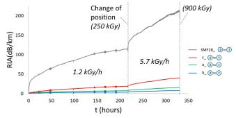
Fig. 2. RIA@1550 nm vs. time for fibers a, b, c and SMF 28 during irradiation 1/configuration " 2to ". The dose rate is 1.2 kGy/h before the change of position and 5.7 kGy/h after. At the change of position, the cumulated dose is 250 kGy, at the end of irradiation, it reaches 900 kGy.
