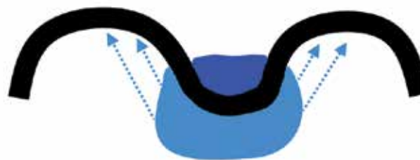
Figure 2. Illustration of irrigation in water furrow wicking into soil beds where rice is growing.
