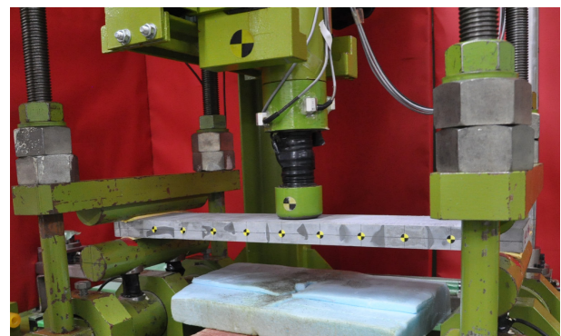
Fig. 6 Setup of impact-loading test.
