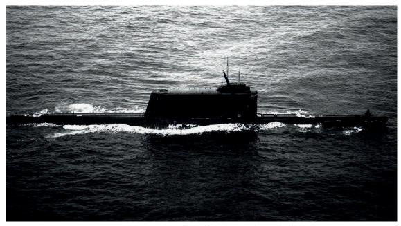
Fig. 16: Like its Hotel-class nuclear counterpart, the Golf-class carried three ballistic missiles in its elongated sail. After the switch to longer-range missiles and a much larger, Western-style missile battery in the Yankee, these early ballistic missile submarines were reassigned to the theater nuclear strike mission. (U.S. National Archives)
