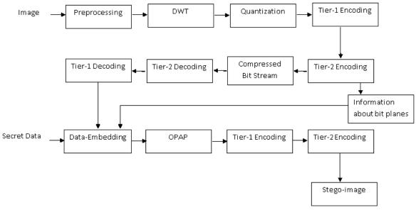
Figure 2. Flowchart of proposed technique using BPC
