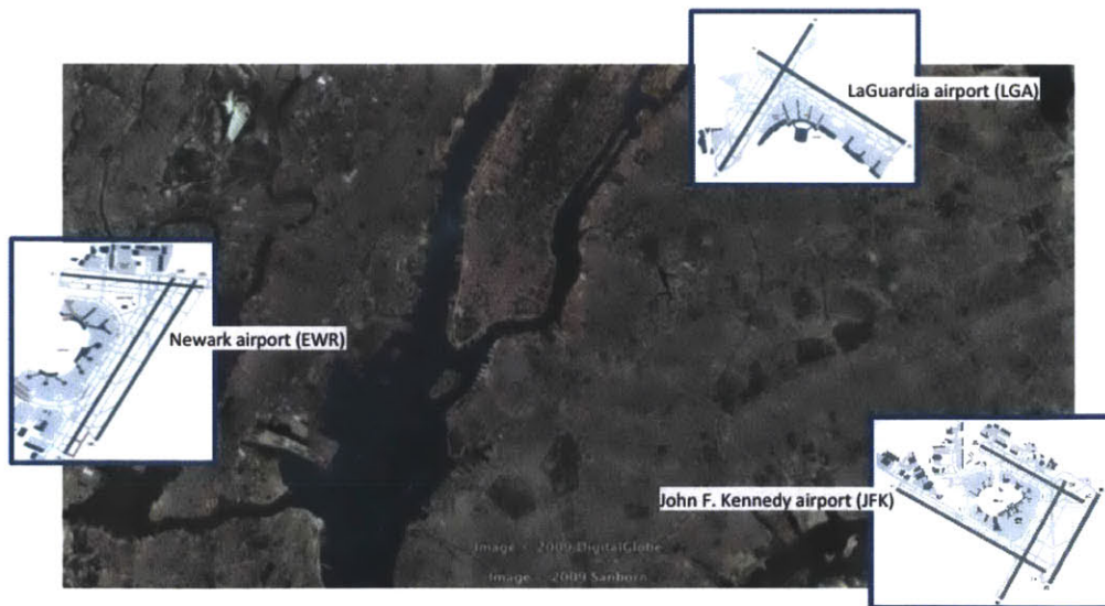
Figure 2-6: A map of the New York area, showing the approximate locations of the three core airports and their relative layouts. Note that the airport layouts are not to scale with the map. © Google. Image © 2009 DigitalGlobe. Image © 2009 Sanborn.
