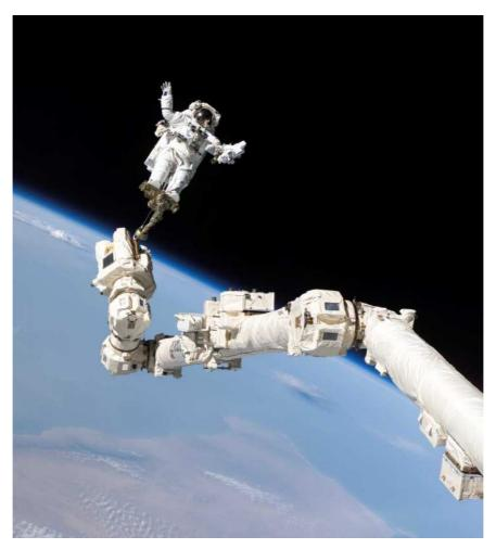
Figure 1.1 – An astronaut attached to the end effector of the SSRMS.
