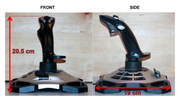
The RHC, shown above, had a range of rotational motion of about 20 degrees in each direction, with an approximately linear spring constant requiring the following forces at maximum displacement of the approximate center of grip (~10 cm from the pivot point, which is visually obscured by the rubber gasket):
