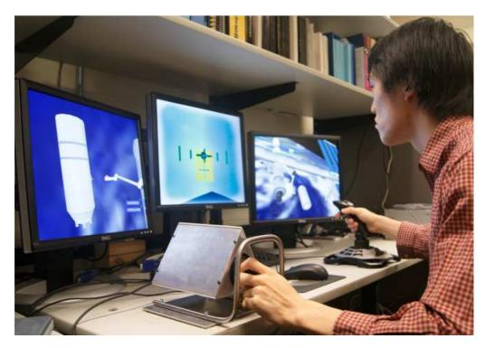
Figure 4.5 – A photo of the RWS simulation environment, showing the THC, RHC, and camera view screens. The central view screen has been photographically enhanced to show the target alignment markings.
