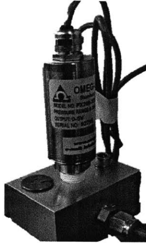
Figure 11: The pressure sensor used during valve testing, Omega model PX209-300G5V
