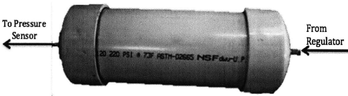
Figure 10: Short section of PVC pipe with end caps. This tank was filled with water and acted as the accumulator tank in the test setup.
