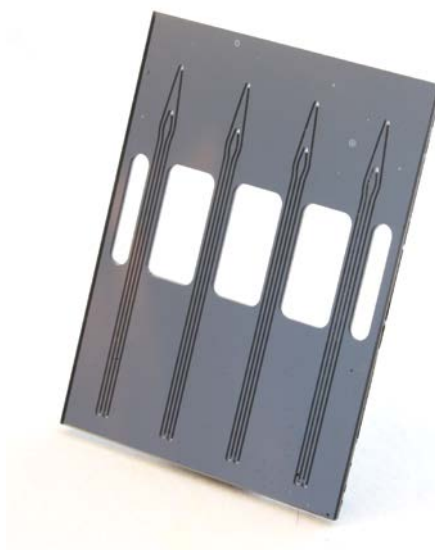
Figure 2.16. Eight channel, four inlet reactor for studying high-pressure gas phase heterogeneous catalysis. (Photo courtesy of Barış Ünal)
