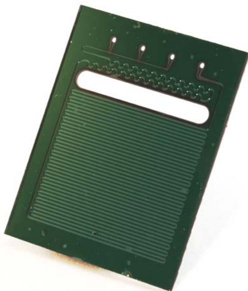
Figure 2.11. Completed homogeneous microreactor.
