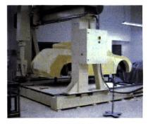
[1.9] C-tek's CNC 5-axis milling machine produces fullscale car models.
