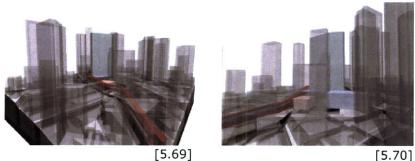
Modelling the design in digital form becomes a very crucial step when the tower begins to take shape. Numerous study models are created on the computer using AutoCAD 2000 and Mechanical Desktop 5 to design, represent and evaluate the surface structure of the tower.
