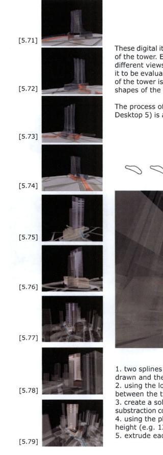
These digital iterations demonstrate the form-making process of the tower. Each study model is rendered in several different views, with or without the site context, in order for it to be evaluated. As mentioned earlier, the phyiscal model of the tower is modelled first in digital form, and then the shapes of the floor slabs are cut using the lasercutter.
