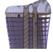
[7.1] This section shows the expansion of floor slabs on the top of the composite tower.
