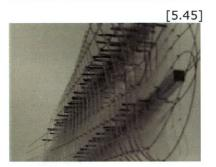
tower structure model: plexiglas, brass tubes, stainless steel wires scale: 1" = 32'
