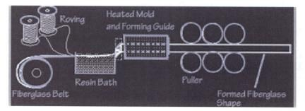
[2.10] the pultrusion process diagram
