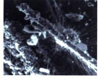
[2.5] A microscopic image of a FRC section shows how relative sizes of fiber and cement. The type of fibers, the volume percent, the orientation and the aspect ratio of the fiber will affect the tensile strength of the reinforced concrete.
