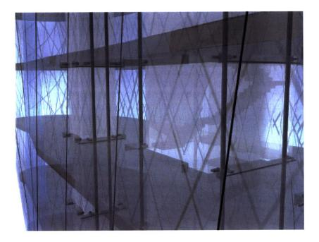
[5.92] This perspective shows the interior component at the core of the tower. While each floor slab is supported by a set of composite cables that goes around the interior up to the cores, a number of roller/damping joints are fastened at the connection between the core and hole of the floor slab to allow for some flexibility.
