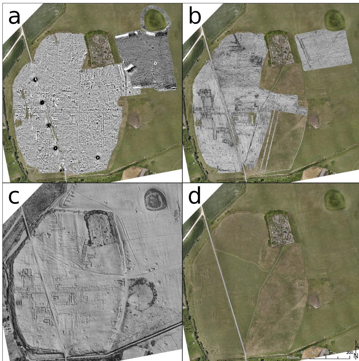
Figure 10. Archaeological prospection data of the central area at Bassianae . (a) Magnetic data image with greyscale values of -6 nT (white) and +6 nT (black); (b) GPR depth-slice from approximately 1.0 to 1.2 m depth; (c) multidirectional hillshade of the DSM with 3 \times Z exaggeration; (d) orthophotomosaic of all UAS images. In contrast to the 1935 aerial photo depicted in Figure 3a, the orthophotograph shown in (d) does not reveal all surface undulations. These are only visible from the air through the proxy of shadow marks. However, the 2014 aerial sorties were not solely flown during low-slanting sunlight conditions (as those of Figure 4) because the DSM offers many ways to visualize these topographic differences.
