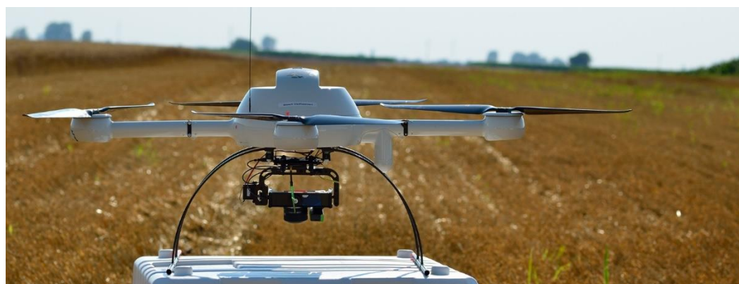
Figure 7. The md4-1000 quadcopter with a Sony NEX-5N mounted in a small carbon fibre camera mount on site. Photo: Geert Verhoeven.
