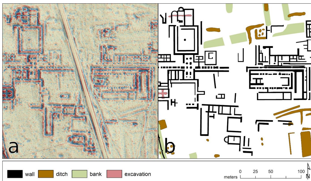
Figure 12. (a) Detail of a fused DSM visualization: a simple local relief model (circular kernel with 40 cells radius, (-0.15 m, 0.15 m) clip, blue-yellow-red colour map) merged with a multidirectional hillshade ( 35^\circ solar elevation, vertical exaggeration factor of 3) using two iterations of the “hard light” blending mode with varying opacity levels. The contrast of both source layers was slightly altered before the initial blending. (b) Corresponding archaeological interpretation.
