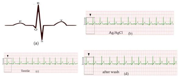
**Figure 1.** (a) components of ECG signal, (b) signal collected using Ag/AgCl electrode, (c) signal collected using textile electrode, and (d) signal collected using textile electrode after washing. All signals are collected in static conditions.
