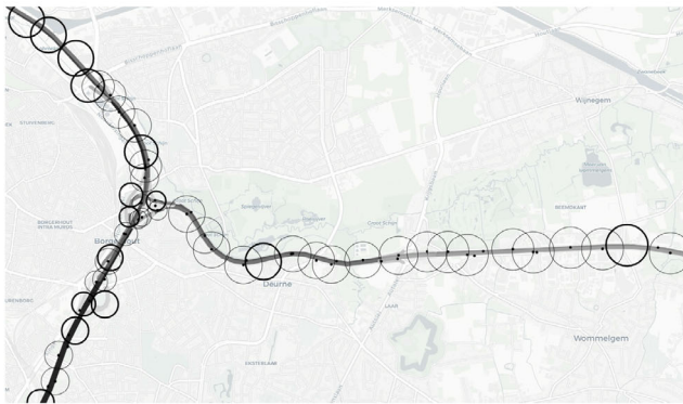
(a) Selected RSU locations within the pilot site, for average traffic density and the default range of 350 metre. Bold circles represent new RSUs, normal circles upgraded RSUs. Existing cabinets are shown by the black dots. The darker the highway segment, the higher the average traffic density on the segment
