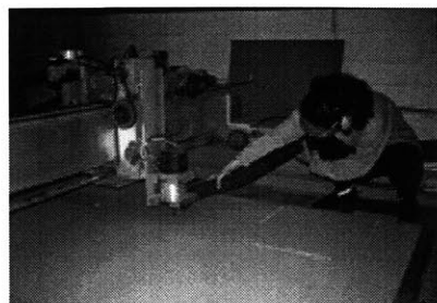
Fig. 9 CNC router cutting the chair
