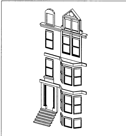
Figure 3-25: Level 3 and 4 components of the rowhouse facade
