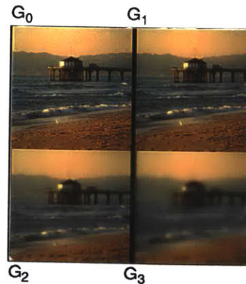
Figure 10. An example of an expanded pyramid. G_0 is the original, G_1 - G_3 show the expanded pyramid levels.
