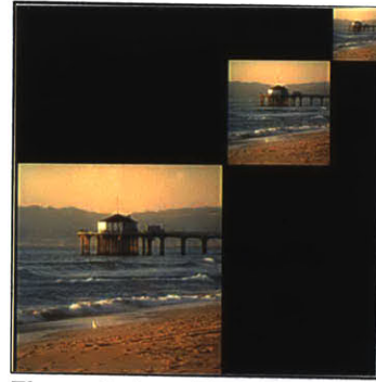
Figure 9. An original image and two levels of its corresponding pyramid, decreasing in size by a factor of two.
