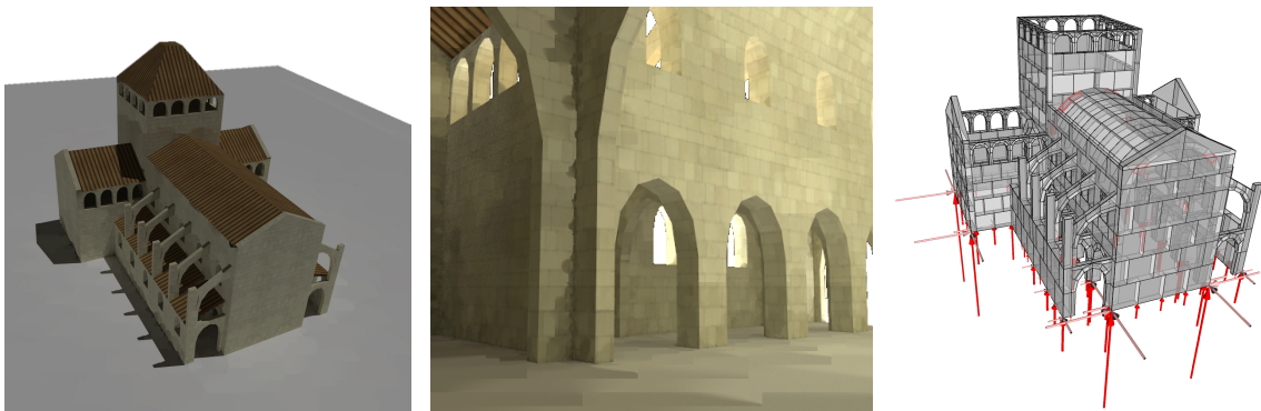
Figure 4-1: Our method generates models of masonry buildings that are structurally stable. In this building based on Cluny Abbey in France, parameters controlling the flying buttresses, columns, and window sizes have been automatically optimized to support a stone barrel-vaulted ceiling. The right image shows reaction forces at the ground plane. We solve for forces at all block interfaces, and apply a compression-only constraint for masonry materials.
