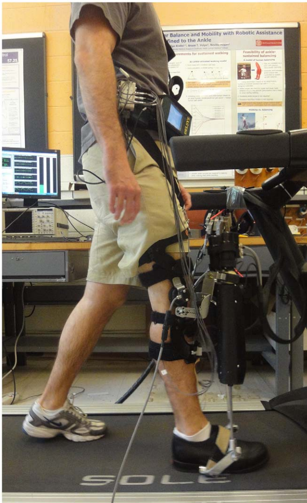
Figure 1. An unimpaired human subject wearing Anklebot while walking on a treadmill. doi:10.1371/journal.pone.0031767.g001
