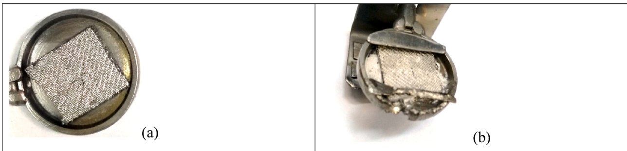
Fig. 4. Tin capillary-porous system: (a) before testing, (b) after plasma irradiation in the PLM.
