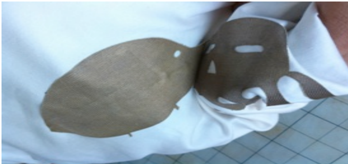
Fig. 4 Pillow's switch recording. Patches of conductive fabric designed after the "dream creatures" of a 9 y.o. girl
