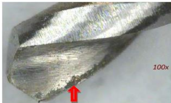
Figure 4. Twist drill edge chipping type of wear at lip. 85
