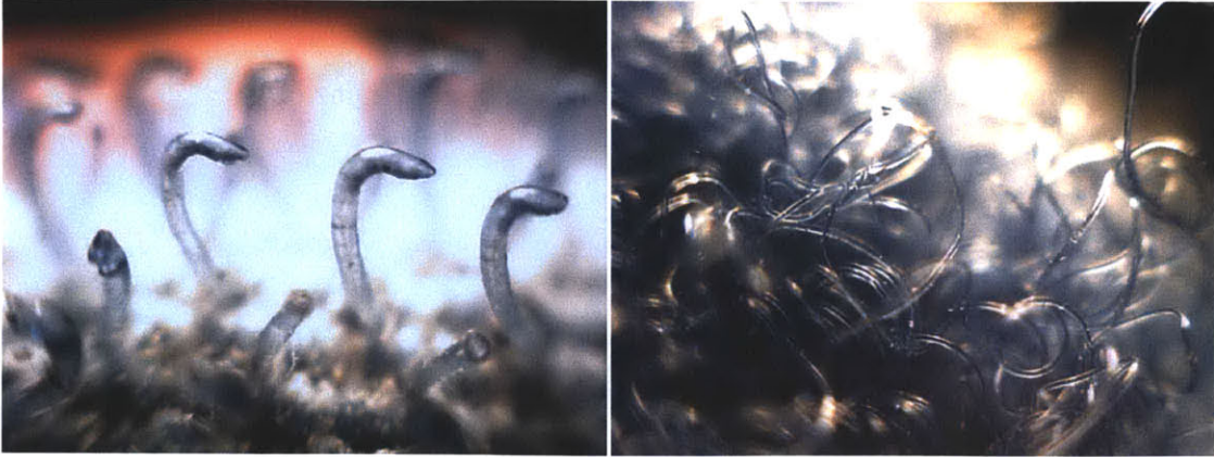
Figure 1: Photos of Velcro hooks (OLIVEPIXEL, VELCRO HOOKS) and loops (OLIVEPIXEL, VELCRO LOOPS).
