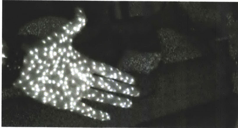
Figure 4. Infrared Dots Projected by PrimeSensor
