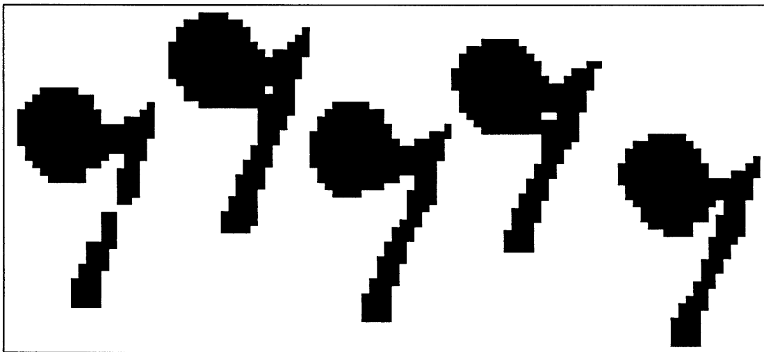
Figure 3-2: Because of quantization noise and printing irregularities, the same feature doesn't always have the same pixel representation.
