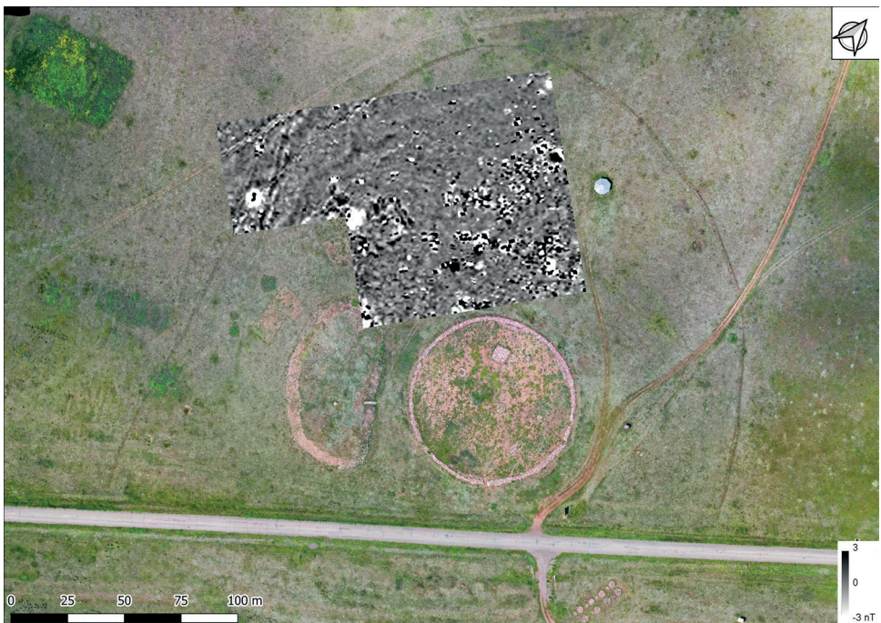
Fig. 6. Turan-Uyuk valley. Surroundings of barrow Arzhan-2. Magnetic map, anomaly range of -3/3 nT, greyscale, overlaid on orthophoto
