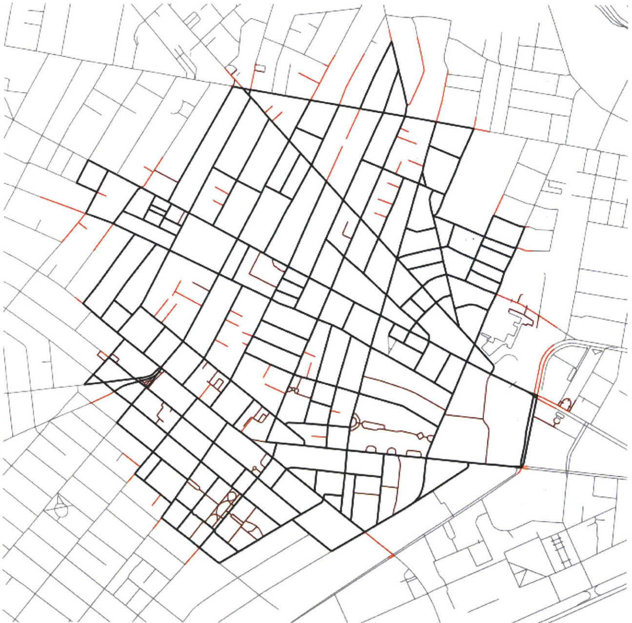
Figure 5.4: The map server processes street data to match a request from the iPhone client. Starting with a center point, unnamed streets (dark red) and streets that are too far away (gray) are removed from the data set. Then all the dead ends (red) are dropped, resulting in a clean and fully connected subset of streets (black).
