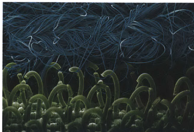
Figure 1: The hooks and loops of Velcro are able to grip upon contact, much like burdock burrs snag on to the fibers of hair and clothing. [1]
