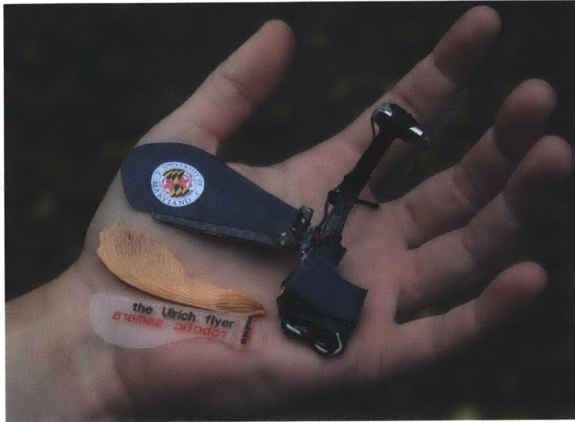
Figure 3: At-scale robotic maple seed developed by Ulrich et al. [5]
