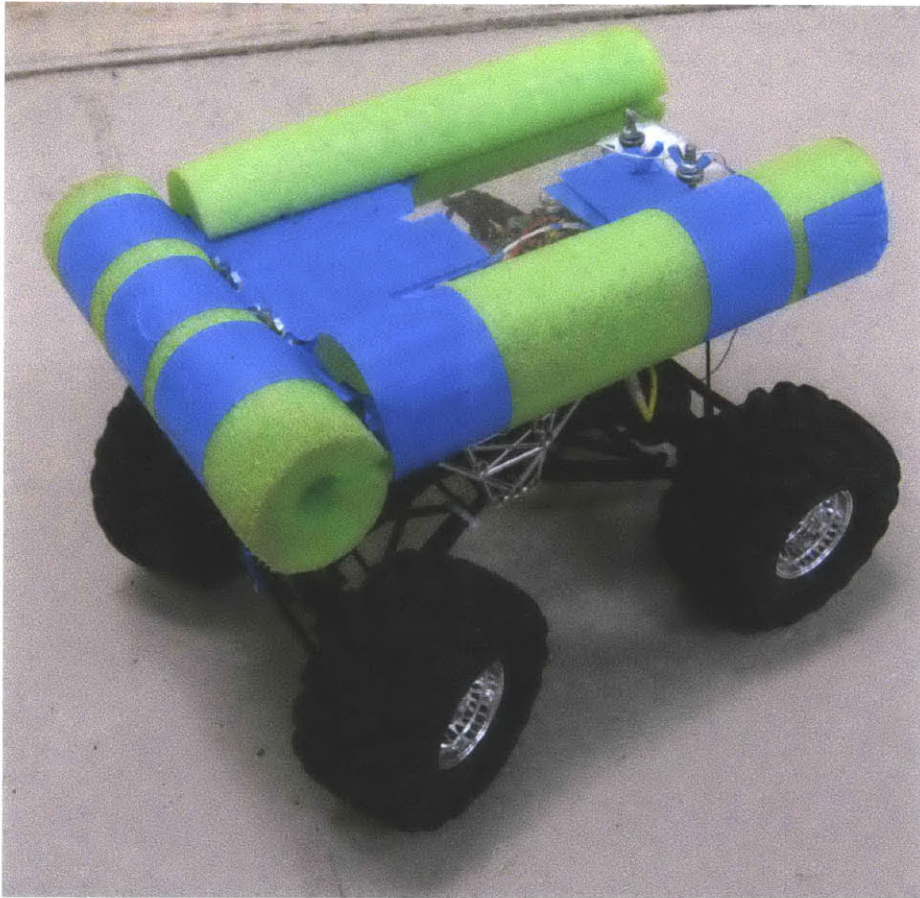
Figure 4: The robot used in the study. The sides have been padded with foam to cushion the vehicle during rollover.
