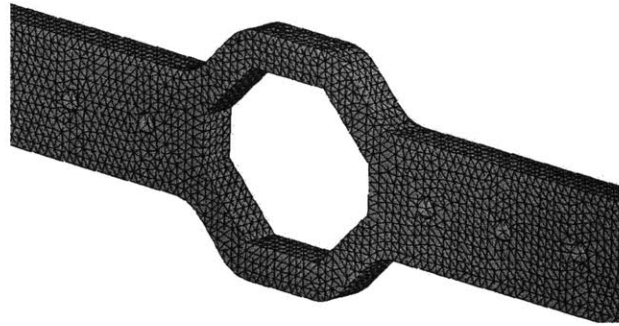
Figure 2-5: SolidWorks Simulation Mesh of 56,564 4-Node Elements
