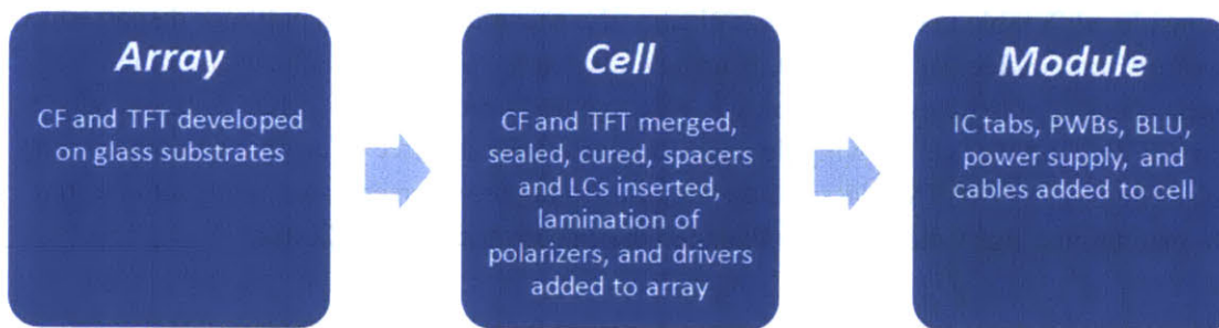
Figure 11. Stages of LCD production as described in literature
