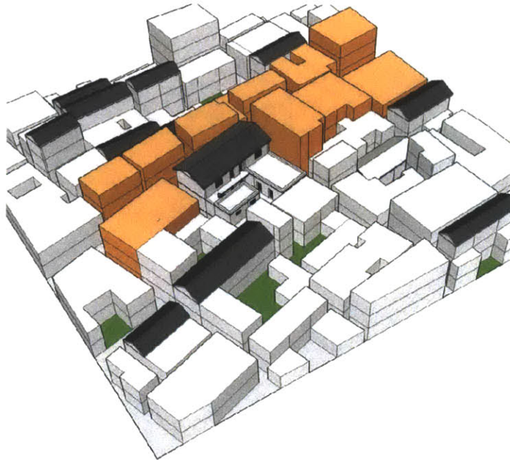
Figure 4.1 The typical traditional neighborhood in Jinan (The model is Zhangjia Village) Source: "Making the Clean Energy City" in China research project, MIT, 2010 Note, the green space is the courtyard, and the orange buildings are commercial facilities.
