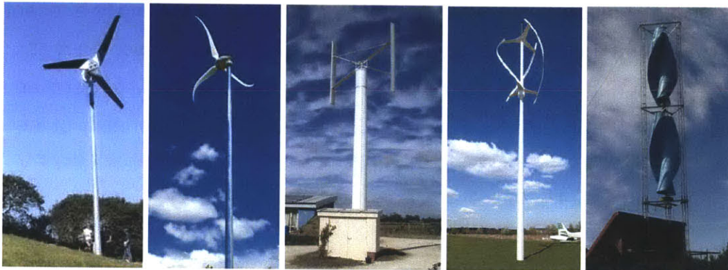
Figure 2.4 Different types of wind turbines, from the left to right are Proven Turbines (HAWT), Skysteam 3.7 (HAWT), QR5KW triple helix blade (VAWT- Darrieus), Skyrota 5.0 two blade (VAWT-Giromill), Helical 3 KW wind generator (VAWT-Savonius) Source: http://www.solener.com/novedad_e.html (the first right) http://www.planetenergy.co.uk/windtubines_files/ (the others)
