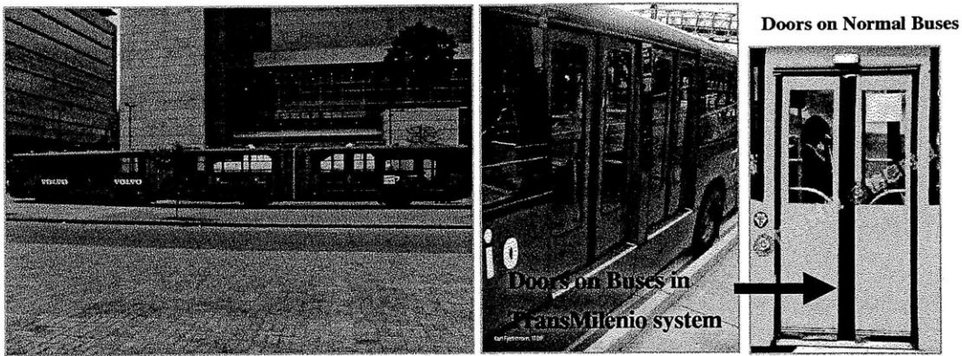
Figure 2.1-7: The vehicle and the double two-sashed doors in TransMilenio system
