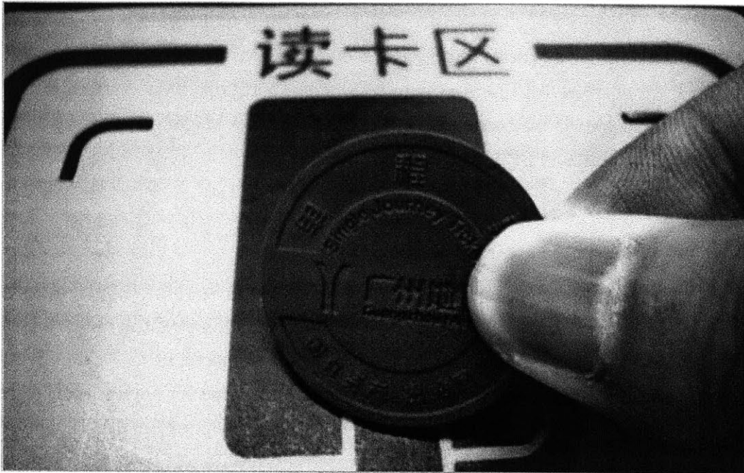
Figure 4.3-10: The new magnetic token (one-way ticket) used in Guangzhou metro Source: [http://www.gzlive.net/bbs/thread-27996-1.html]
