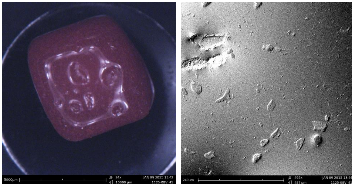
Figure 10: Optical micrograph and SEM image of glass sample, Orange 1125-08, with 2-hydroxyethyl cellulose as a binder. Fired embedded in vermiculite at 730°C maximal temperature. The SEM was taken at 500x magnification.
