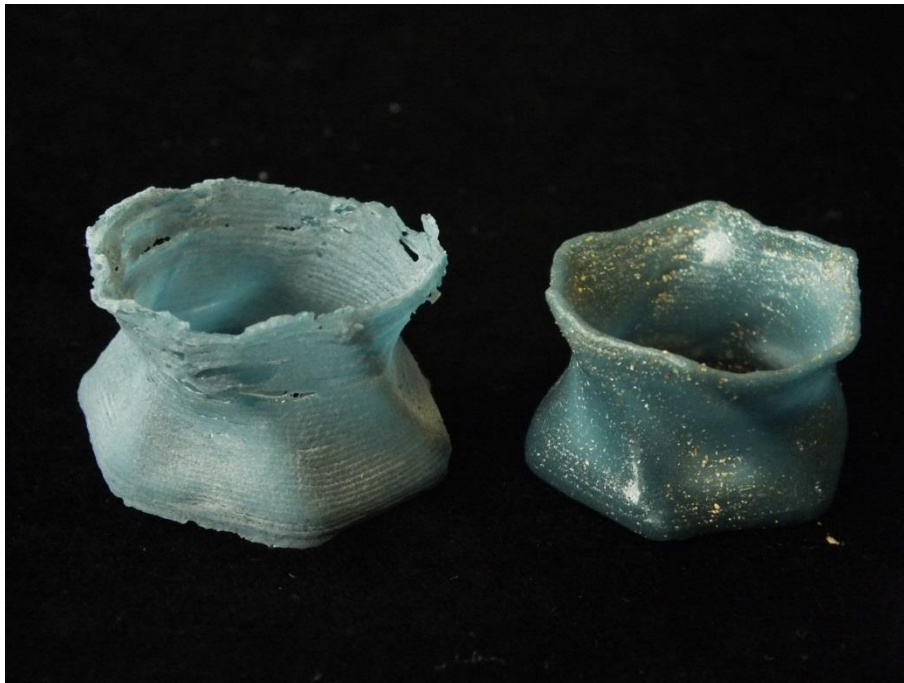
Figure 7: Direct printed objects. The different surface finish is the result of different support materials during firing. On the left side plaster was used. On the right side vermiculite was used.
