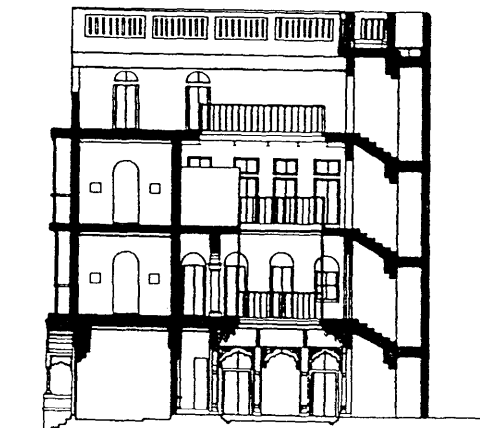
[3.67] Individual buildings occupying the full extent of the lots and organized around a central courtyard
