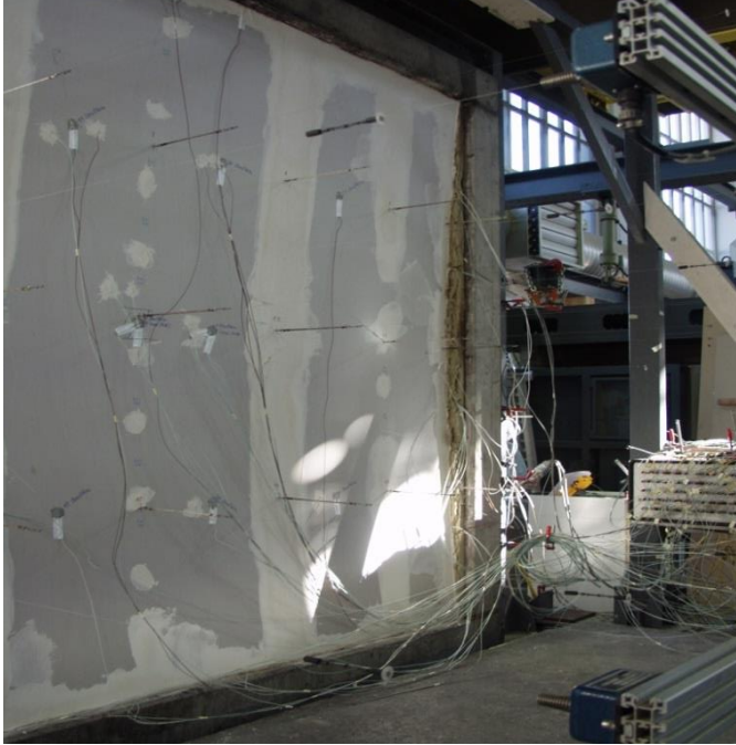
Fig.4. The test wall after bowing into the fire (one hour exposure).
