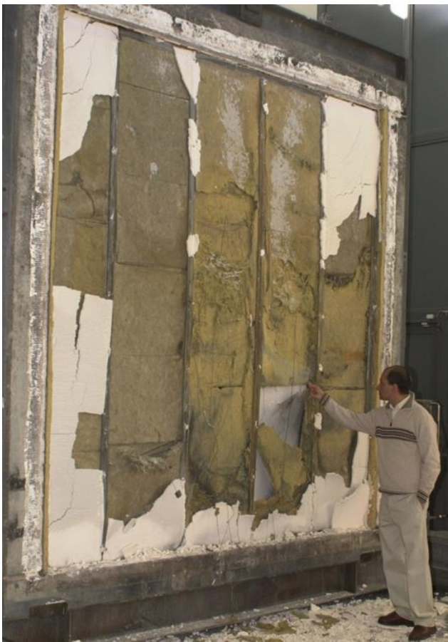
Fig.7. Post-fire examination of the test wall
