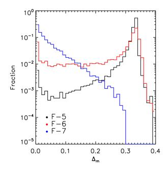
Fig. 1.— Distribution of  $\Delta_{\rm m}$  (=  $M_D/M_L - 1$ ) for different  $f_{R0}$  models as labeled on the figure. A galaxy is less screened for large  $\Delta_{\rm m}$ . A fully unscreened galaxy has  $\Delta_{\rm m} = 0.33$  (higher values are due to simulation inaccuracies). As we move from the F5 to the F7 model, fewer halos are unscreened – though a significant fraction still show small deviations, i.e.  $\Delta_{\rm m} < 0.1$ .
