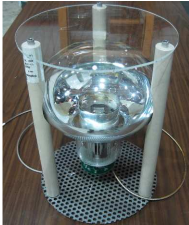
Figure B-3: MicroBooNE PMT supporting frame mock-up, made of three 1-inch diameter grooved PEEK posts surrounding the PMT in at three equidistant positions.
