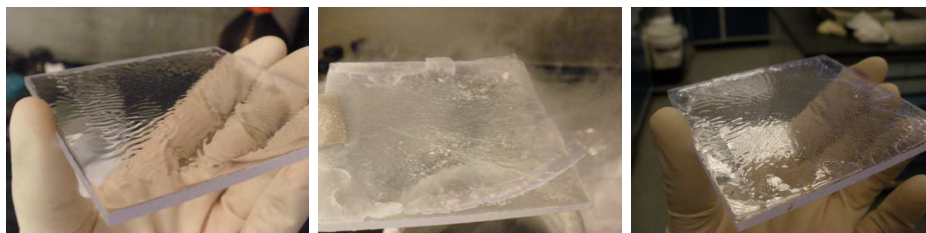
Figure B-19: Testing of TPB-PS drip-coated acrylic plates in liquid nitrogen. Acrylic sample coated with TPB-PS before immersion in liquid nitrogen (left); immediately after immersion (middle); and an hour after immersion (right). The TPB-PS coating detaches from the acrylic surface near the edges of the plate, and visible cracks form across the full surface of the coating. The plate itself shows no signs of cracking.
