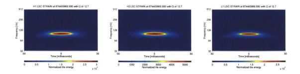
Figure 7-22: Sine-Gaussian f=100 Hz Q=9 hardware injection.
