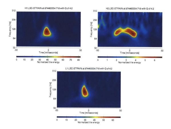
Figure 7-2: Spectrograms of LIGO calibrated strain data for each instrument. Normalized energy Z is related to signal-to-noise  $\rho = \sqrt{2Z}$ . Note the different color scales in each plot, and the much weaker signal in H2. The spectrograms are generated over the Q Pipeline tiling [74, 104].
