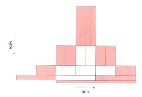
Figure 5-7: Definition of distance from a wavelet coefficient (in white) to other coefficients in the time-scale decomposition. Tiles with a distance of 1 (light pink) and 2 (dark pink) from the original tile in white are shown. A typical distance threshold used for clustering outliers is 2.
