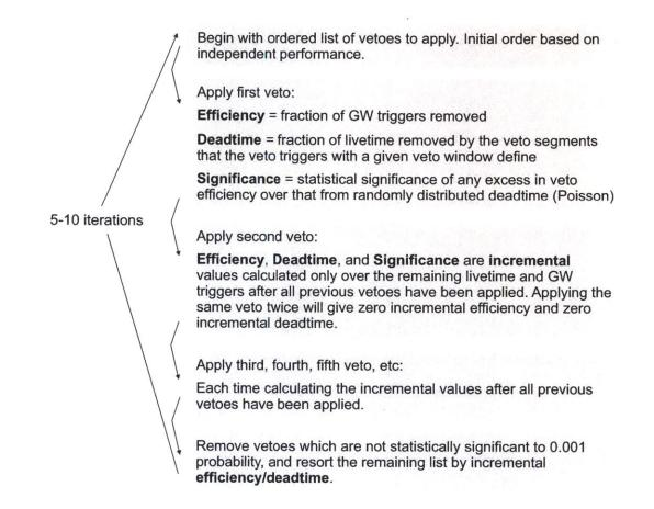
Figure 6-3: Procedure used for ordering a list of veto conditions from best to worst in terms of channel, frequency range, window, and threshold. A set of vetoes can then be chosen for any choice of dead-time threshold by choosing the corresponding top ranked vetoes. The particular method of refining the list order over several iterations is chosen because it minimizes the number of steps which must be done in serial and therefore is easy to implement on a computing cluster.
