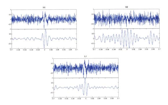
Figure 7-1: Whitened plots of the uncalibrated signal LSC-DARM\_ERR (differential arm length error signal) for each instrument are shown over 60–2048 Hz and a restricted 60–140 Hz band.
