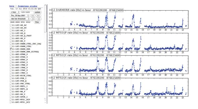
Figure 6-1: Rate of transients vs. time as identified by the kleineWelle pipeline. The rates are calculated every few minutes and available through a web interface. Shown here are correlations at L1 between single-detector noise transient rates in the gravitational wave channel (DARM\_ERR: error signal for differential arm length control) and alignment channel transients from the mirror wavefront sensors.
