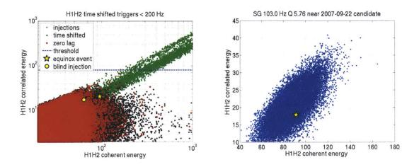
Figure 7-4: Q Pipeline correlated vs coherent energy in the context of expected background (left) and simulated signals (right). The left plot shows the burst event (equinox event) as well as an earlier semi-blind inspiral injection. The equinox event falls within the expected parameters for both all burst simulated signals (green bar) and specifically the closet match sine-Gaussian simulation (blue cloud). Black dots on the left plot show the population of sample time-shift background.
