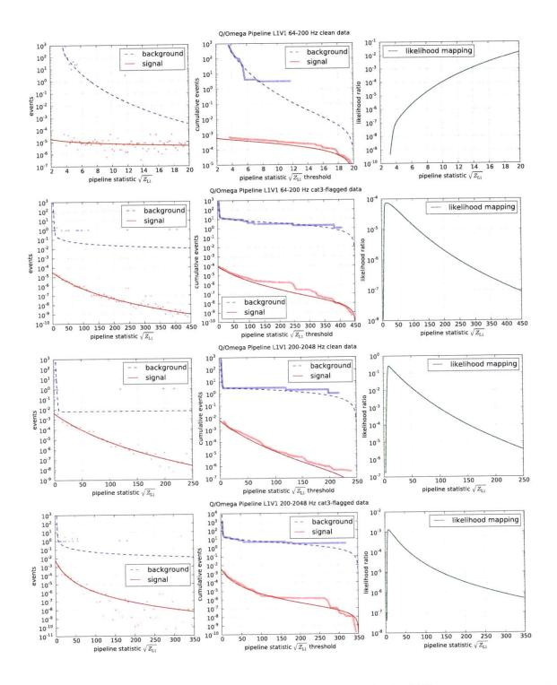
Figure 8-5:  $Q/\Omega$  Pipeline L1V1 likelihood-ratio maps Dashed blue curves represent the population of sample background events from 1000 time-shifts. Red curves represent the number of signals from the single homogeneous mock population, scaled appropriately to the number of time-shifts and relative bin size (for the case of the discrete histogram). Analytic fits to the discrete distribution are used to calculate the likelihood-ratio mapping (signal/background) for the configuration.
