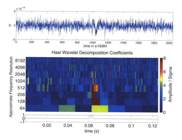
Figure 5-6: Decomposition of a  $\sigma = 1$  ms Gaussian injection with match filter signalto-noise ratio of 11 onto simulated LIGO S2 noise. Shown at top is the signal+noise after high pass filtering at 50 Hz and LPEF whitening. Shown at bottom are the normalized Haar discrete wavelet decomposition coefficient amplitudes for the whitened data along with a timeseries of the original unfiltered signal.
