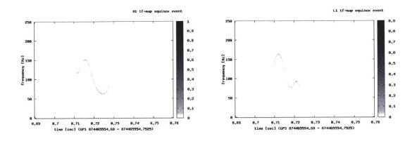
Figure 7-17: The Hilbert-Huang transform of the candidate event indicates a decrease in frequency from about 160 to 60 Hz in just a couple cycles.
