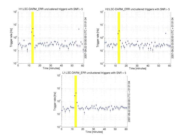
Figure 7-6: Q Pipeline trigger rate vs. time during the hour of the event which occurs at 3:06 UTC. The rate is for non-overlapping (in time-frequency) triggers with SNR > 5 prior to 1 Hz down-selection. The event occurs during an increase in H1 trigger rate. The yellow bar marks a series of hardware injections.
