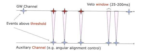
Figure 6-2: Simple veto logic used by auxiliary channel event-by-event vetoes for S5. A channel-specific veto window is constructed around the central times of auxiliary channel triggers above a certain threshold (represented as gray stars on the bottom time-line). Gravitational-wave channel events are removed (red stars) if their central time falls within the veto window. The veto procedure removes a small amount of live-time from the analysis.
