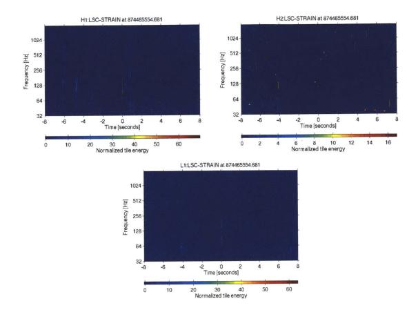
Figure 7-5: Plots showing Q Pipeline single-interferometer non-overlapping triggers in time-frequency space in  $\pm 8$  s of the event time. H1 shows a large number of weaker transients in the immediate neighborhood of the event.
