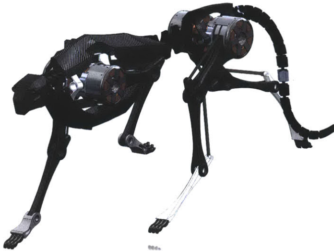
Figure 1-1: Conceptual model of the MIT Biomimetic Robotics Laboratory Cheetah, a high-speed running robot. This thesis presents a high-level control approach for this and other robotic runners
