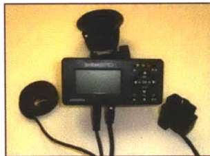
Figure 2.7: Auterra DashDyno (center), GPS Unit (left), and OBD-II Connector (right)
