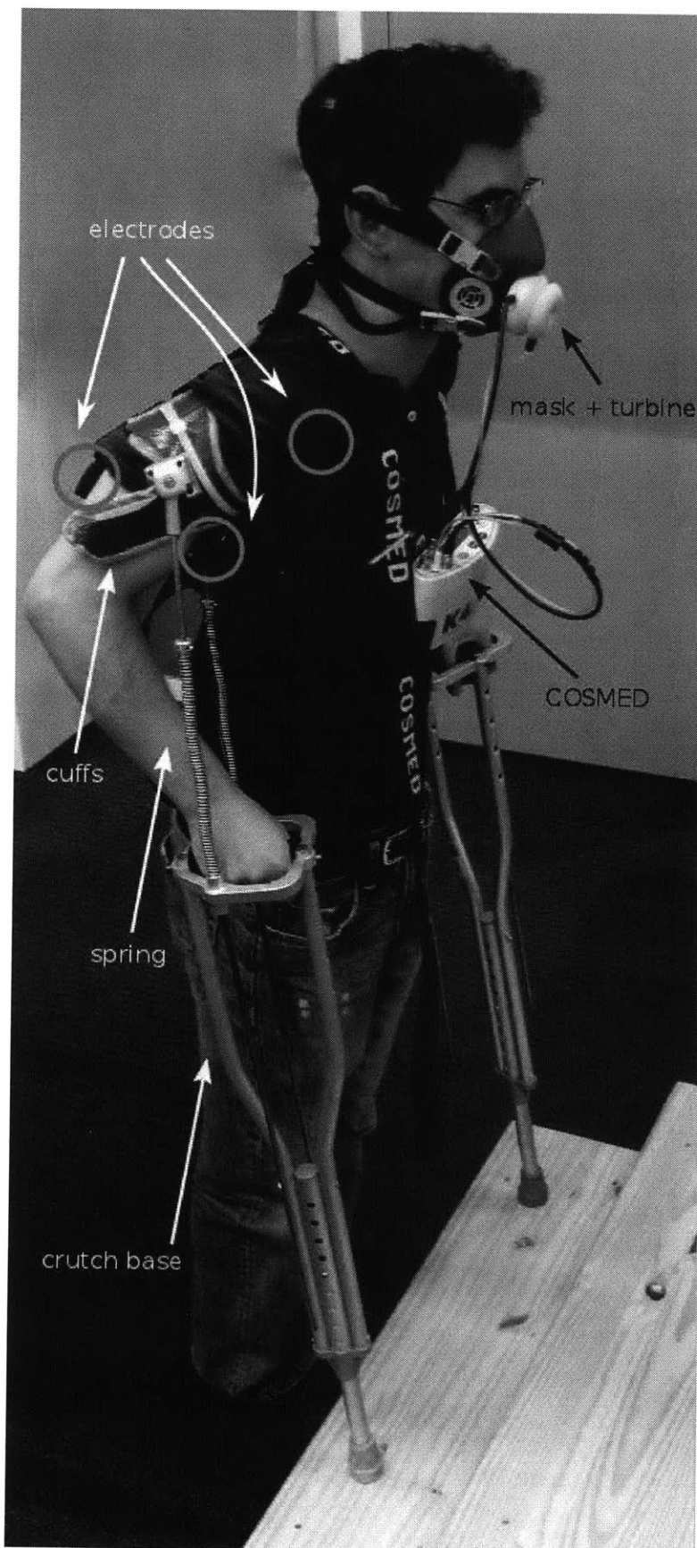
Figure 3-2: Subject crutching up stairs with instrumentation gear. Electrodes locations are circled.
