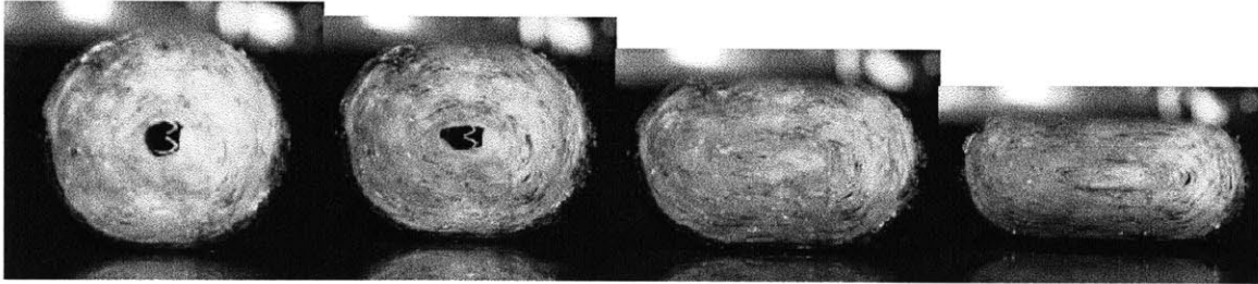
Figure 6: Lateral compression test. Performed with internal jellyroll intact.
