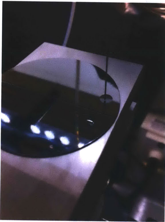
Figure 1-13: 10 microliter water droplets on each side of 50/50 bare silicon and fluorosilane surface. The contact angle on the bare silicon side (top) was 10 \pm 2 degrees, and the contact angle of the fluorosilanized surface (bottom) was 122 \pm 2 degrees. Contact angles were measured on a Ramé-aart Model 500 Advanced Goniometer with DROPimage Advance v2.4 software.
