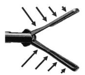
Figure 1: Uneven pressure on current grasper jaws.
