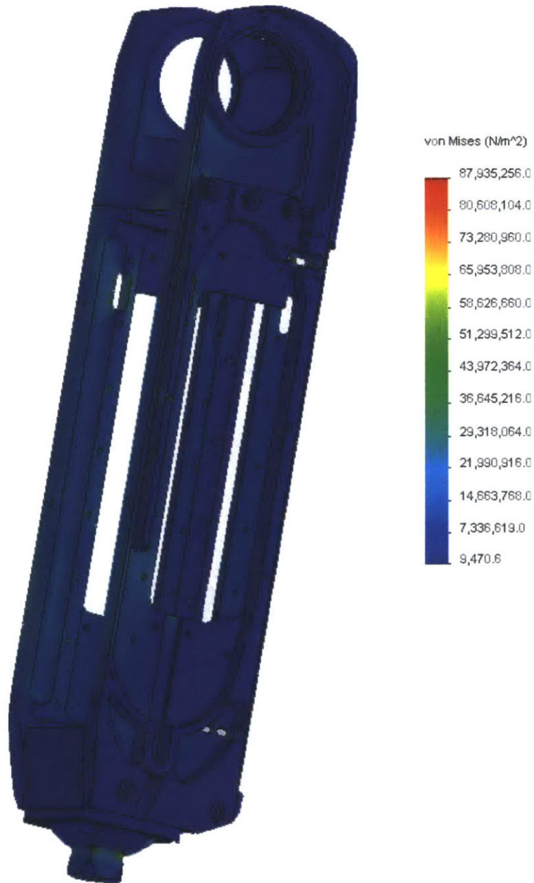
Figure 3-8: Finite element analysis showing the stress distribution of the Revision_1 active knee chassis.
