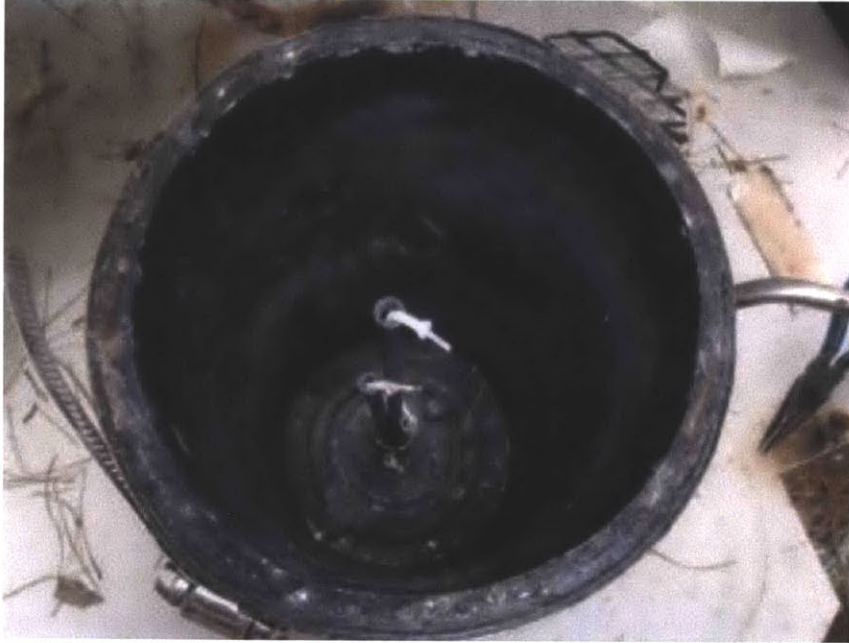
Figure 11: Four thermocouples placed at different heights in the burn chamber
