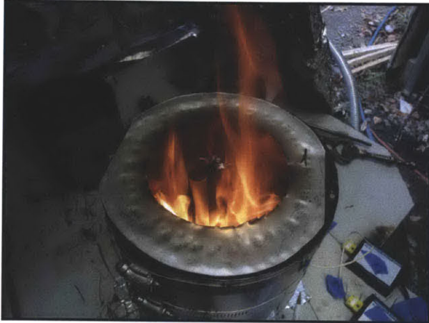
Figure 16.a: Flames. Photo of secondary burning during the testing of Configuration C.
