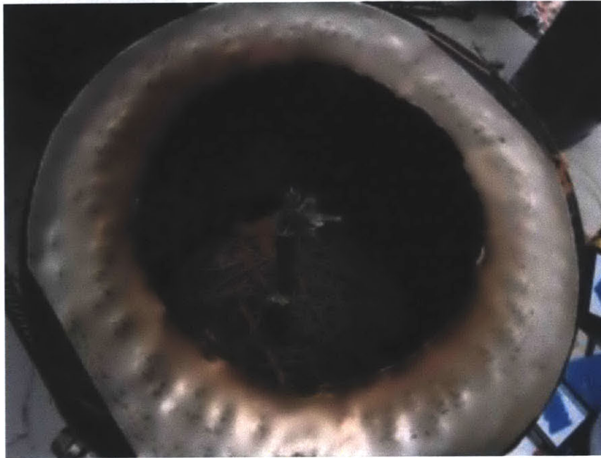
Figure 13: Testing unit as it is being filled with pine needles before a trial. The cylindrical cover was placed over the opening to restrict the draft slightly.
