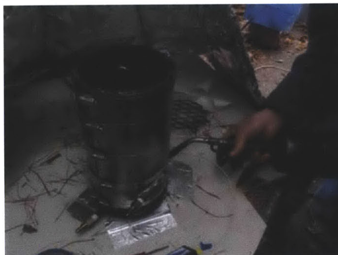
Figure 8: The testing unit underneath a hood. The gas torch was used to light the pine needles.
