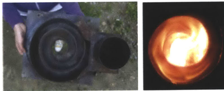
Figure 5.a: Top view of the spiral geometry above the firebox where volatiles undergo secondary combustion through an elongated burn path and high heat from firebox below.
