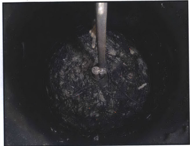
Figure 18.a: Ash Fuel Bed. Photo of the fuel bed after testing Configuration D. Ultimately, all the fuel converts to ash.
