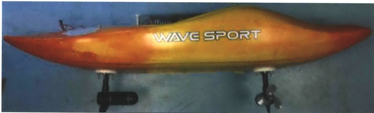
Figure 2.1: Profile of HoverGroup kayak with bow and aft azimuthing thrusters.
