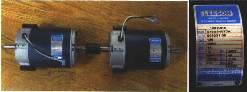
Figure 17: Coupled DC Drive Motors and Specifications
