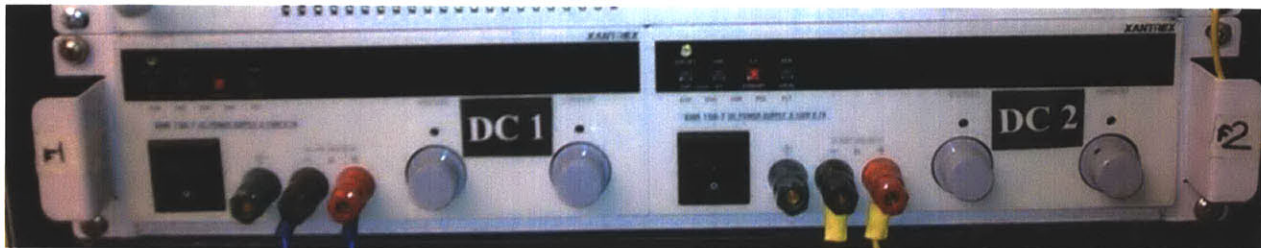
Figure 18: DC Motor Power Supplies
