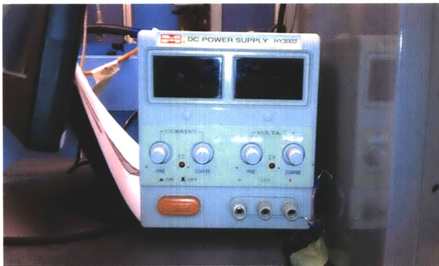
Figure 39: Relay Power Supply (PS2)
